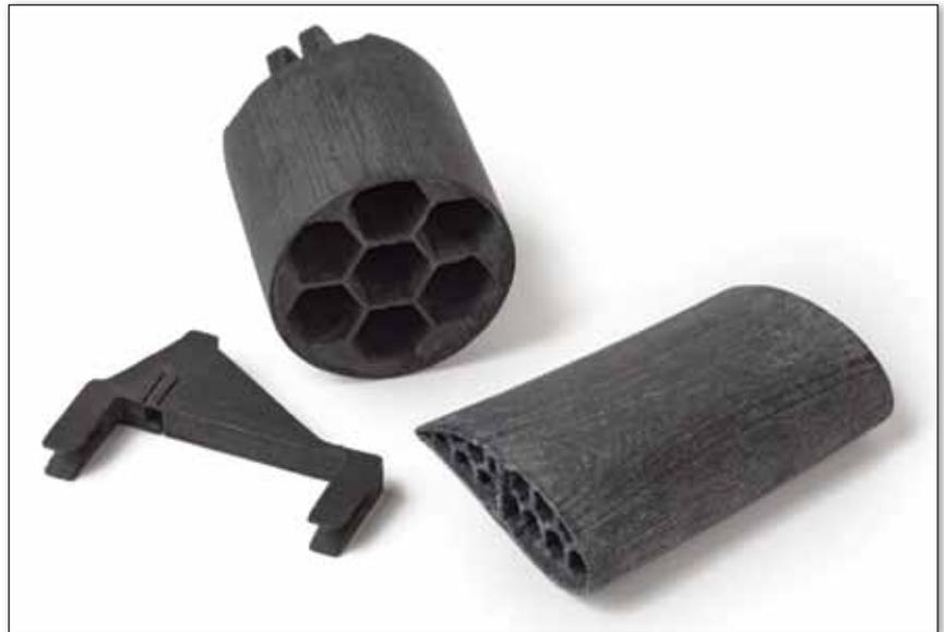
**3D CBAM parts (left to right):** Small aircraft rear stabilizer mount, aerospace clevis strut, automotive air foil.
