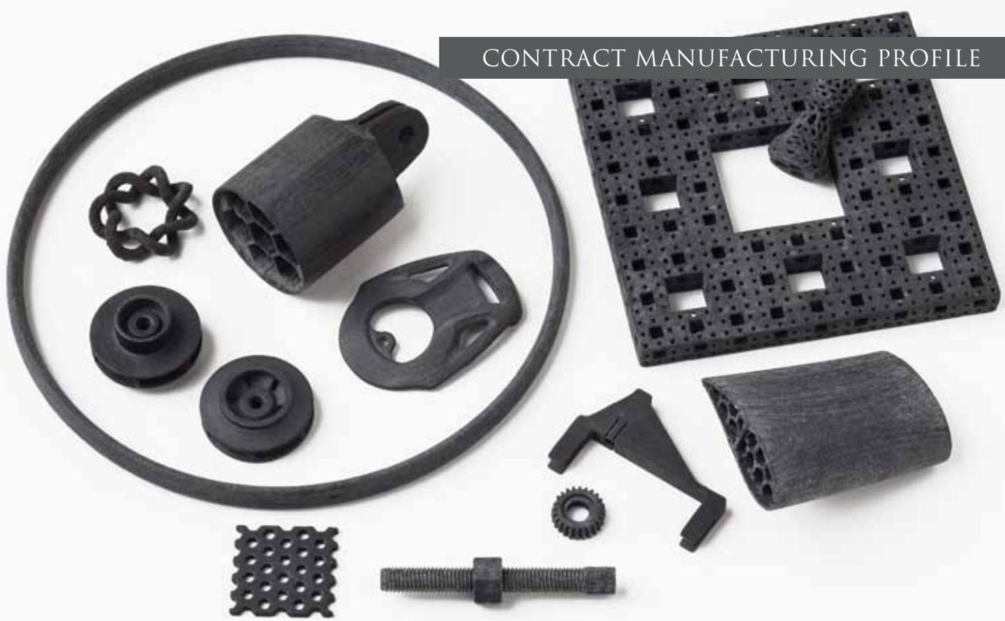
3D carbon fiber composite parts made from Impossible Objects' CBAM process.
