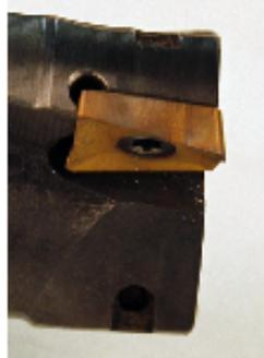
Total Removal Before Tool Failure 315.3 Cu in
