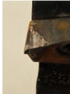
Total Removal Before Tool Failure 93.4 Cu in
