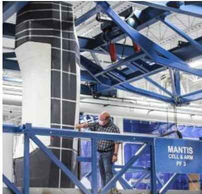
Fuselage Overbraid on Mandrel
