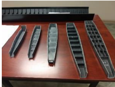
Wing Rib Matched Metal Molds - WiSDM
