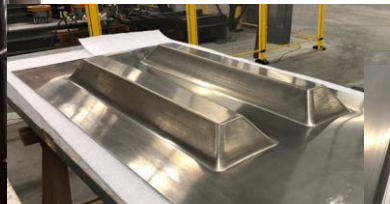
Tools fabricated for : Hat Stiffeners Fuselage Bulkhead Scaled Wing Skin
