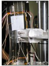
Composite skins **bolted** to **metal** substructure
