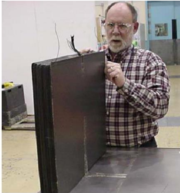
Successful Cure of 3 1/2 inch Thick Laminate First Time - Using Analysis To Specify Cure Cycle
