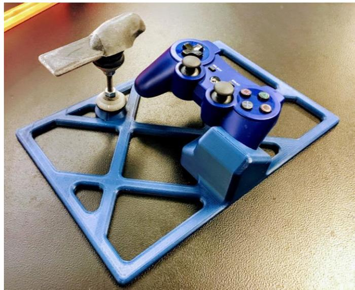
Figure CG-2 - The Testing Rig holds the controller and thumb simulator in place for testing.
