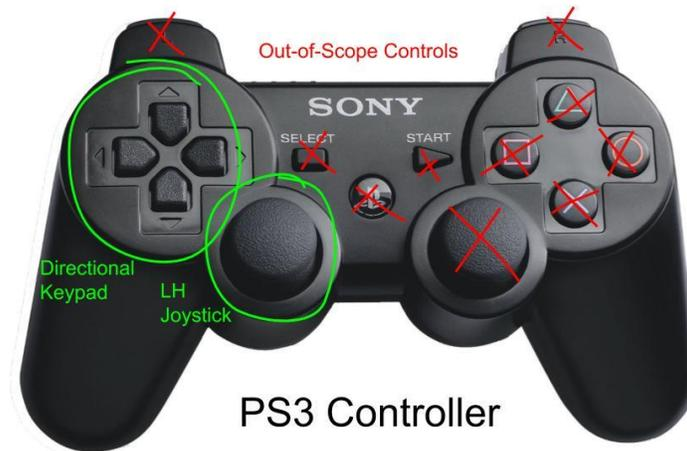
Figure CG-1 - The controls that are circled in green on the PS3 Controller pictured above must be fully operable by the adaptive device. The buttons with red “X”s through them do not need to be operated.
