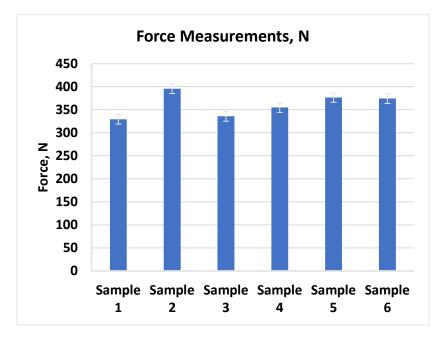
3-point bend test were performed on various 3-D printed gyroid composite panels are shown below
