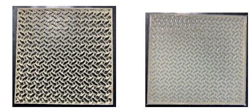
Model structures were printed using Thermoplastic Nylon (polyamide) Gyroid structure with infill epoxy resin as shown below.
