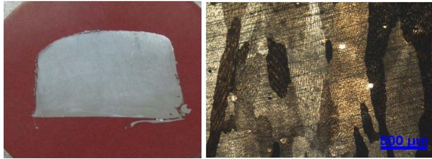
Figure 3. DMD of JBK75 stainless steel. Left: Cross-section of sample deposit. Right: Microstructure.
