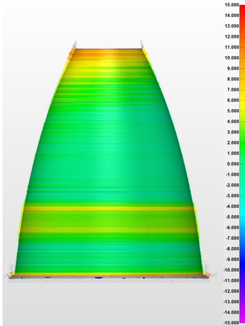
Figure 8. 3D scanned data overlaid on the CAD of the part showing dimensions of the DMD printed part.
