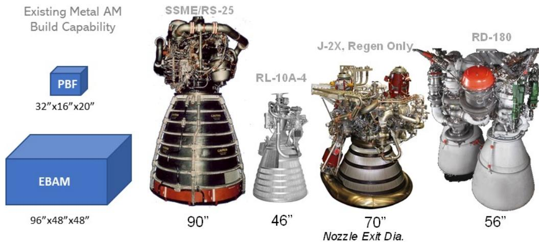
Figure 1. Comparison of current PBF and EBAM machine limitations with rocket engine nozzle needs.
