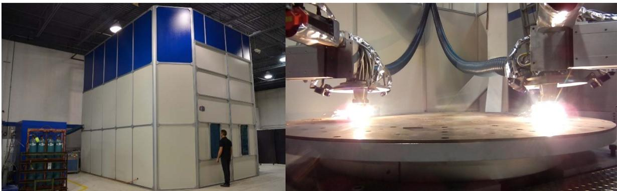
Figure 2. DMD Multi-nozzle system. Left: DMD machine. Right: Dual nozzle technology for rapid 3D deposition.
