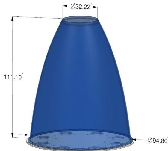
Figure 4. CAD model showing dimensions of the RS-25 engine nozzle liner along with build-plate at the bottom.
