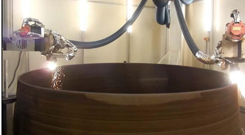
Figure 6. DMD simultaneous dual nozzle printing of the RS-25 liner.
