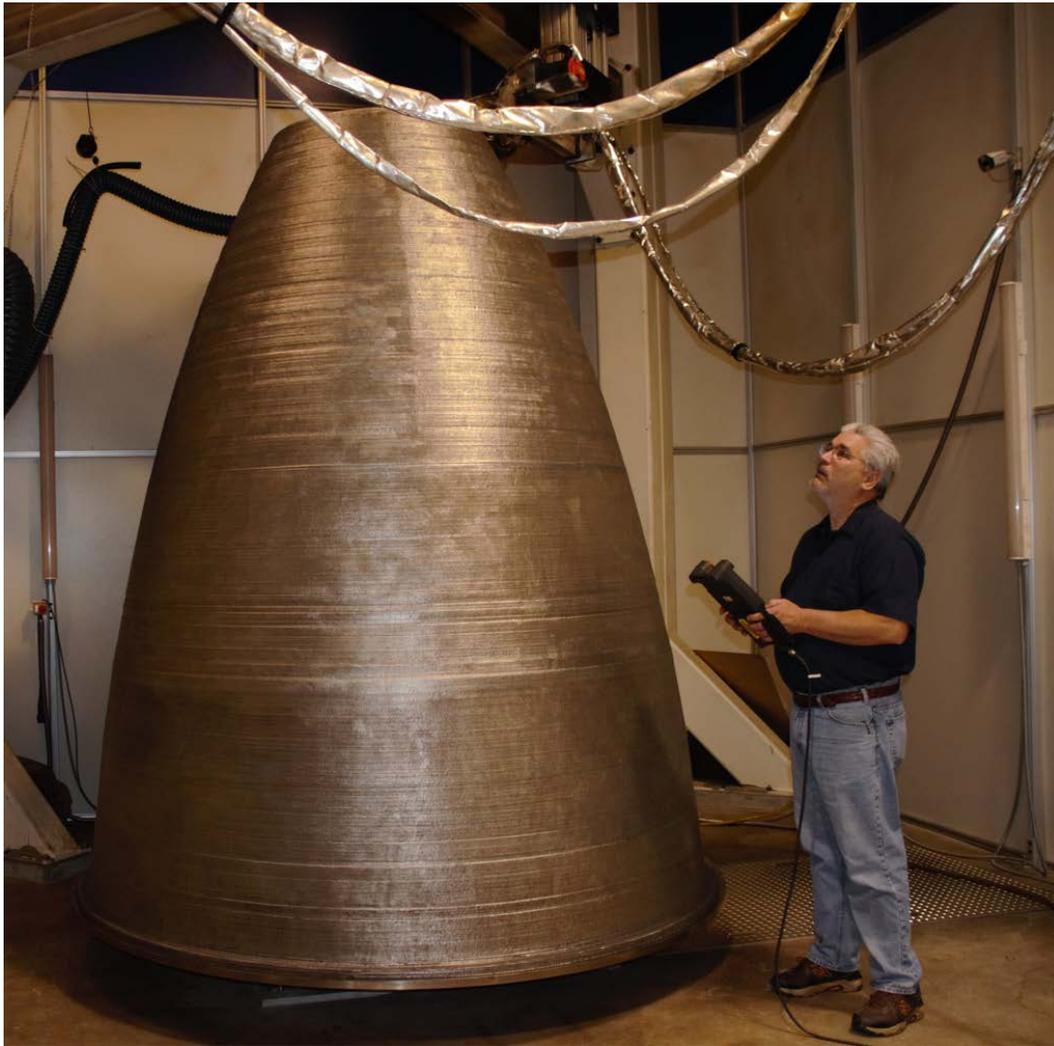
Figure 7. Picture of full-scale RS-25 nozzle liner on completion of the build.
