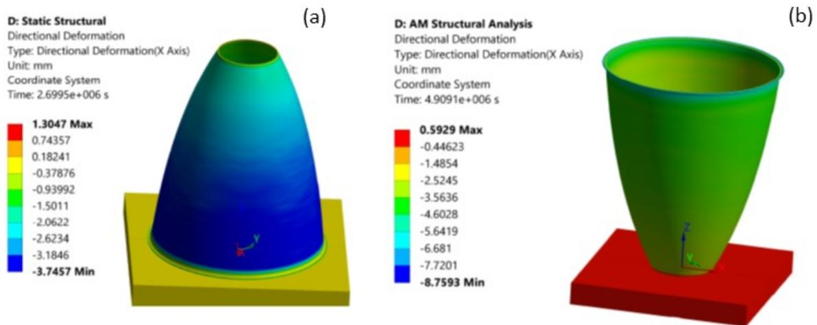
Figure 5. Simulation showing radial distortion of the part in two different build strategies. Left: Bell-end down. Right: Bell-end up.
