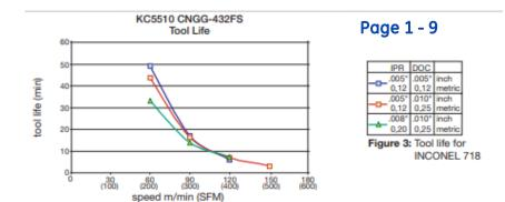
Kennametal PVD coated grade, max. wear (flank, notch) – 300  $\mu m$  , crater wear – 100  $\mu m$
