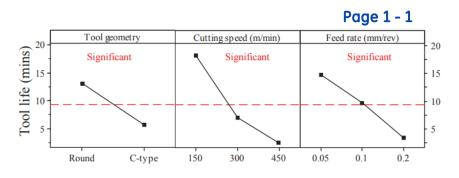
PCBN insert, depth of cut – 0.2 mm, max. flank wear – 300  $\mu$ m, notch wear – 600  $\mu$ m Raw data not published – 27 experiments
