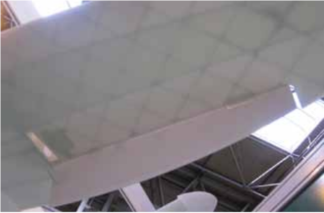
UAV wing with internal ribs for added strength and integrated hinged flap.
