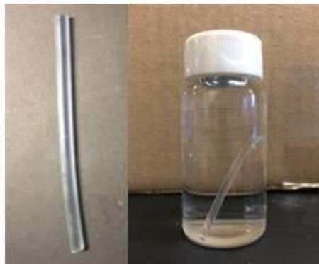
Figure 9: (Left) Sample filament used in water absorptivity test (Right) Set up for water absorptivity test
