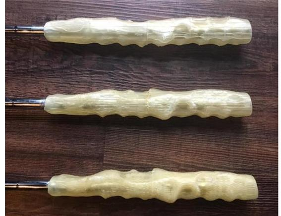
Figure 2: Prototype of golf grips with various infill densities
