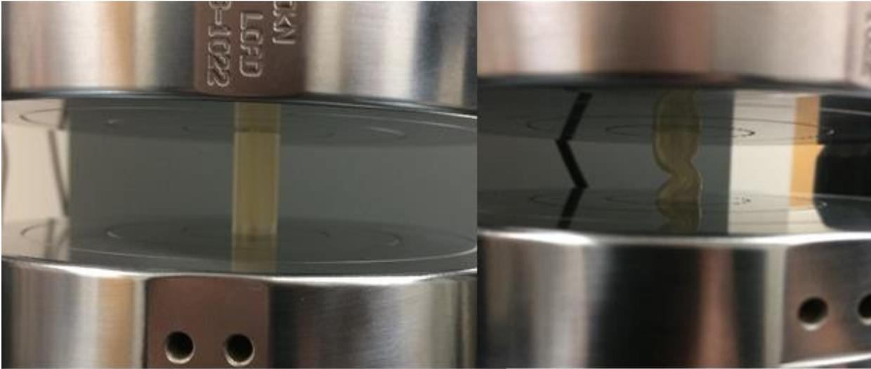
Figure 4: (Left) Compression test with force being applied in the direction of the Z-axis. (Right) Image of buckling failure during axial compression loading of sample
