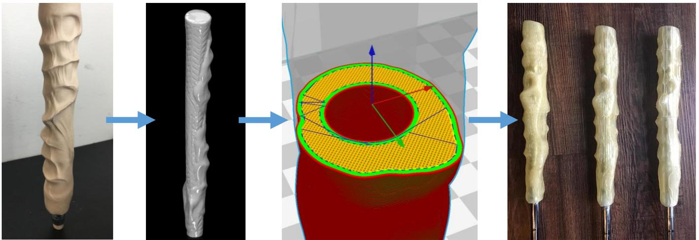
**Figure 1** – Process summary. From left to right: a clay mold is made, an STL is created from the scanned mold, a cavity is added for the shaft, and a set of grips are printed.
