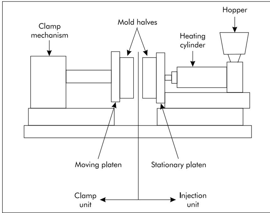
Figure 1-1. The injection molding process.
