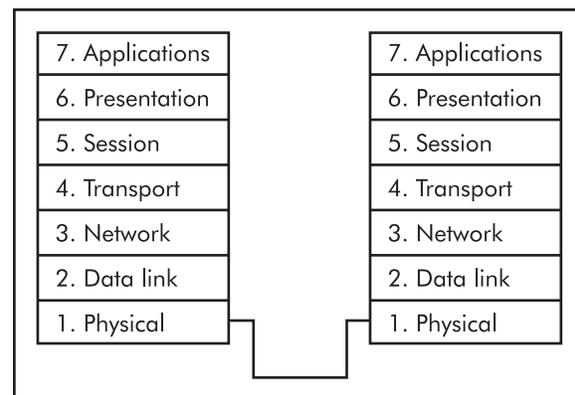
Figure 37-1. Open-systems interconnect (OSI) seven-layer model.
