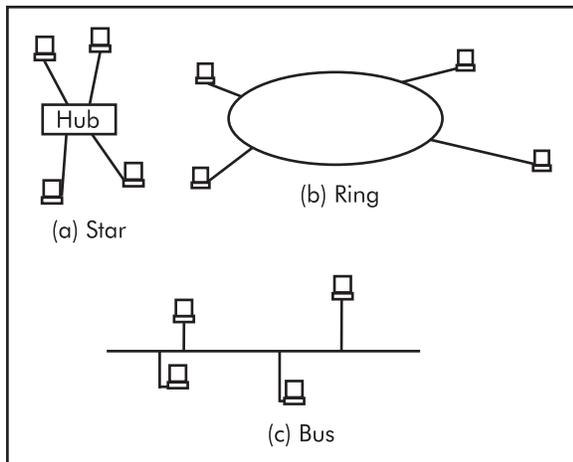
Figure 37-2. Fundamental network topologies.
