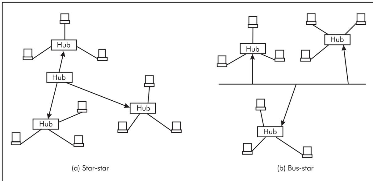
Figure 37-3. Common hybrid topologies.
